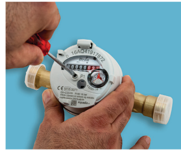
First of all, the plastic piece should be unscrewed from the meter as shown above.
